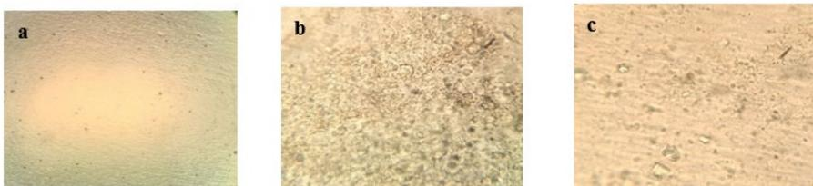
**Figure 2.** Light Microscopic Analysis (1000X) of the LDPE Sheet a) At 0 Hours of Incubation, b) After 40 Days of Incubation, and c) After 60 Days of Incubation
