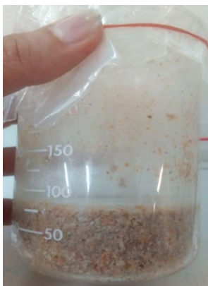
Figure 2. Demineralization and Deproteinization of Chitin
