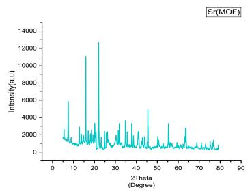
Figure 5. Graphical Representation of Sr-MOF through XRD Analysis
