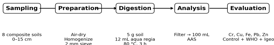
Figure 2. Workflow for Soil Sampling, Preparation, Digestion, and Metal Analysis
