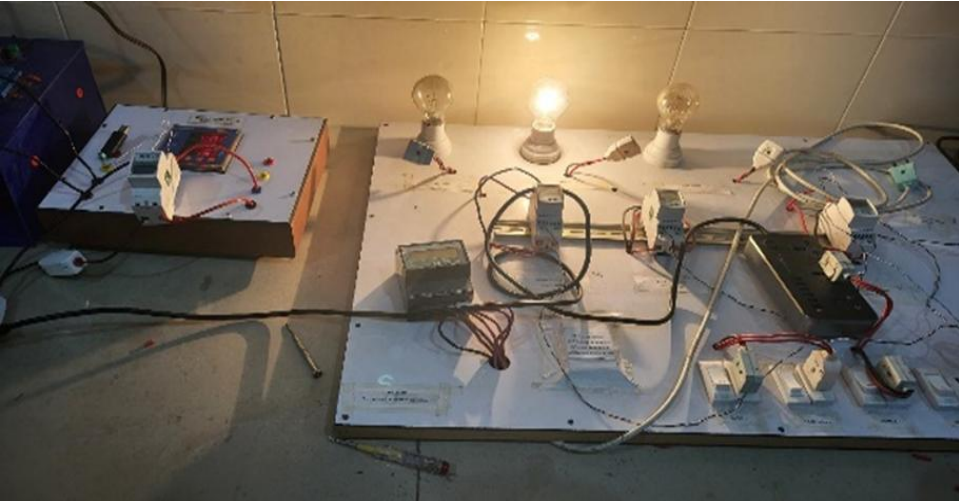
FIGURE 1. SME 104 smart meter collecting data
