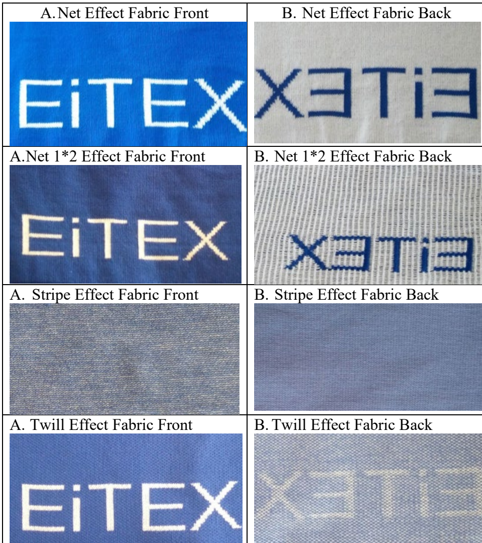
FIGURE 2. Fabric sample of the four jacquard effects on both sides (A. fabric front effect and B. fabric back effect)
