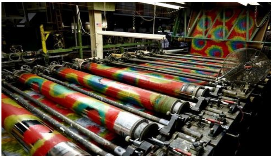
FIGURE 4. Roller printing (fabric)
