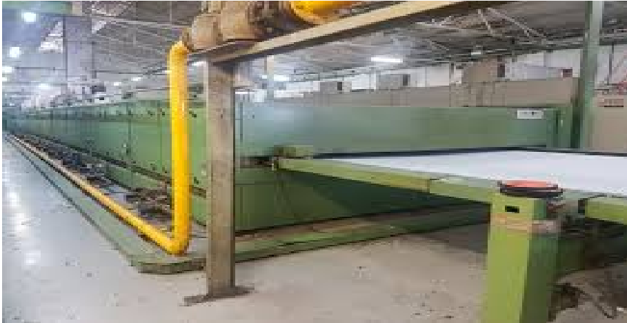
FIGURE 5. Stenter machine for finishing and equalizing processes
