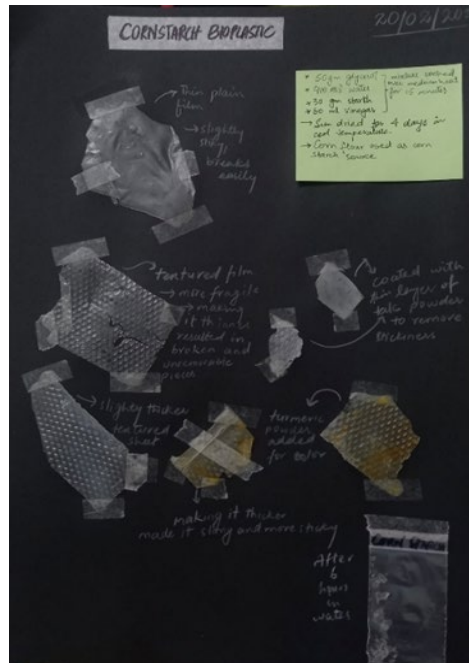
FIGURE 1. Sample # 1 showing experimentation with cornstarch bioplastics, including tryouts with and without textures, colors, and impact of water on it
