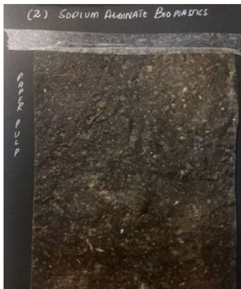
FIGURE 12. Tryout 2, recycled paper pulp in Sodium Alginate bioplastic made as shown in Figure 3.
