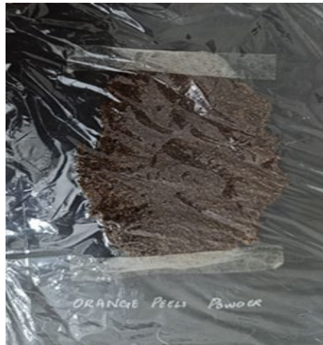
FIGURE 9. Figure 7 orange peels in gelatine bioplastic turned black after 2 months.
